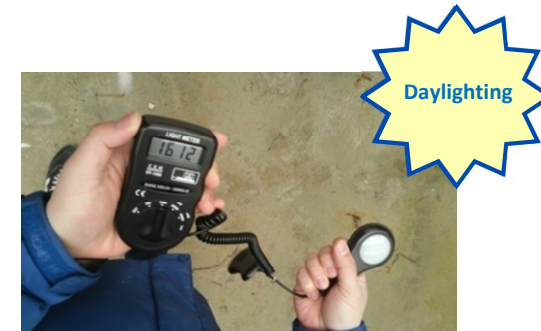
After Deck Installation: 1,612 lux (Fluorescent Light 20W approximately 150 lux)
