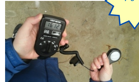
After Deck Installation: 1,612 lux (Fluorescent Light 20W approximately 150 lux)
